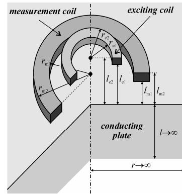
Fig. 1. Coils over conducting plate
