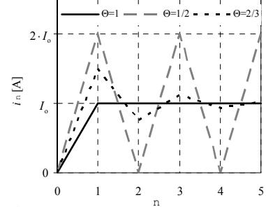
Fig. 4. The discretized excitation of adjoint model for first five time steps and different values of  $\Theta$
