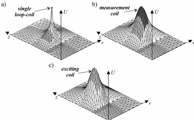
Fig. 3. Modified vector potential  $U$  distributions on adjoint models.
