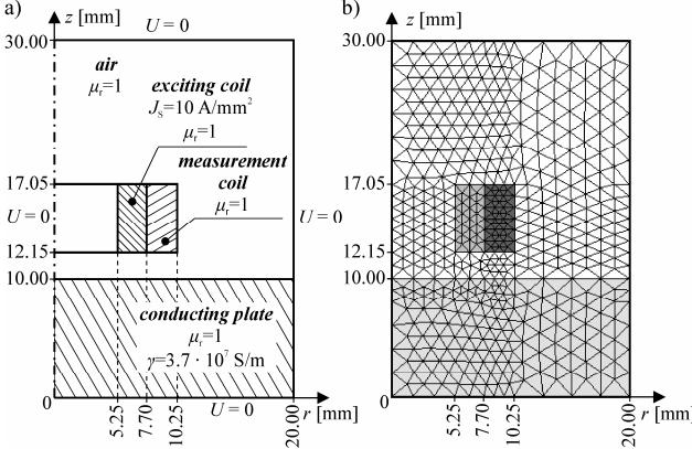
Fig. 2. a) Analyzed model, b) finite element mesh
